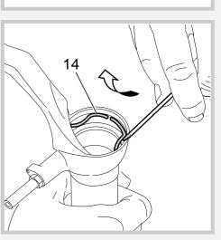
Fit the slider protector **(A)** onto the slider and remove the oil seal **(15)** with the help of a large screwdriver.
